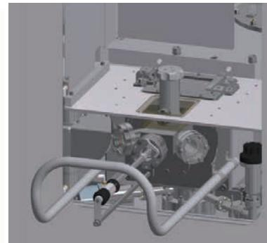
Transfer vessel and transfer vessel adaptor
